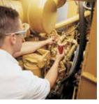
Coolant compartments with sampling valves can be sampled using the same steps as the oil sampling valve method described earlier.
