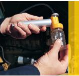
Install a new sampling bottle on the vacuum pump and insert the end of the tubing into the oil - do not allow the tubing to touch the bottom of the compartment.
