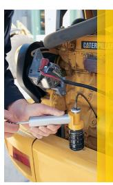
Pump the handle of the vacuum pump to create a suction effect. Hold the pump upright - if you turn it over, oil may contaminate the pump. If oil enters the pump, disassemble and clean it before taking the sample.
