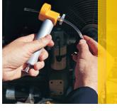
Insert the tubing through the head of the vacuum pump and tighten the retaining nut. The tubing should extend about 4 cm (1 in) beyond the base of the vacuum pump head.
