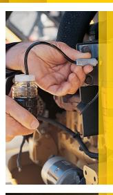
Insert the probe into the valve again and fill the sample bottle half full. Close the bottle cap, shake it vigourously and then dispose the oil once again. Dispose of the used oil properly. This operation is to clean the sample bottle with the sampled compartment used oil. Re-fill this same sample bottle three-quarters full – do not fill to the top. This step will be your oil sample. Do not allow any dirt to enter the bottle or bottle cap.
