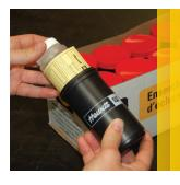
Withdraw the tubing from the compartment. Remove the bottle from the vacuum pump and secure the cap on the bottle. Then place the bottle with the **thoroughly** completed label into the shipping cylinder.
