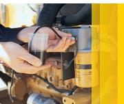
Insert the probe into the valve and collect about 100 ml (4 fl oz) of oil into a waste container. If the oil flow is slow at low idle, it may be necessary to have someone accelerate the engine to high idle while extracting the sample. Dispose of the waste oil properly (This process cleans the valve and helps ensure a representative sample.)
