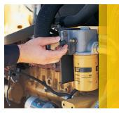
Set the engine at low idle and remove the dust cap from the valve of the compartment you are sampling.
