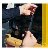
Turn off the engine. Measure and cut new tubing to the length of the dipstick. If the compartment you are sampling does not have a dipstick, cut the tubing so that it reaches about halfway into the oil depth.
