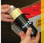
Withdraw the probe from the valve and secure the bottle cap. Then place the bottle with the **thoroughly** completed label into the shipping cylinder.
