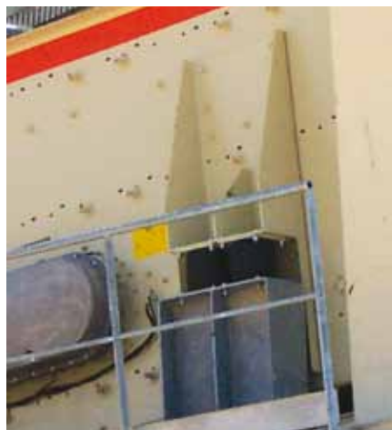
Cordspring rubber suspension.
