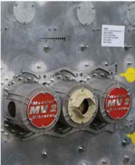
Vibrators synchronized by gears.
