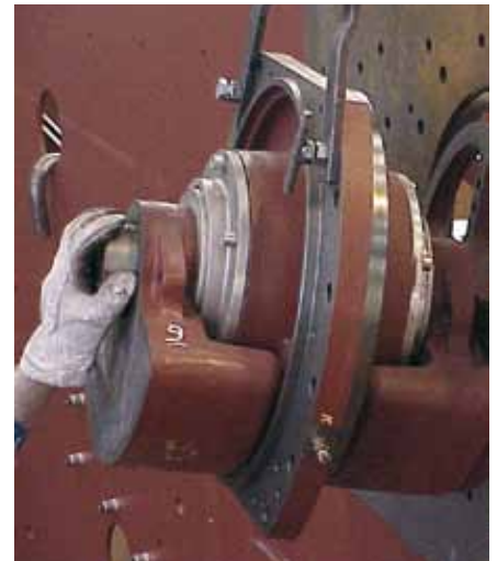
MV vibrator installation.
