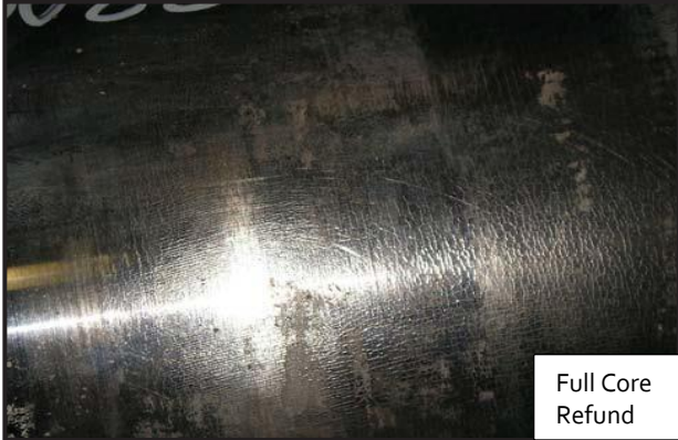
Figure 1: Spider web cracking on rod chromed surface.
